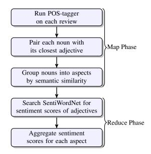
Figure 1: Block diagram of the Semantic-based Approach for Aspect-level Opinion Mining.
