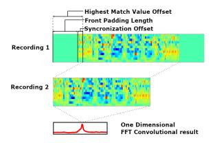
Figure 2: Synchronization between two recordings
