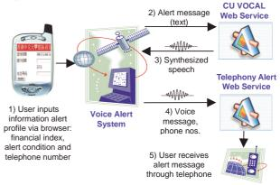
Figure 2. System architecture of the CU VOCAL voice alert system that integrates several Web services.
