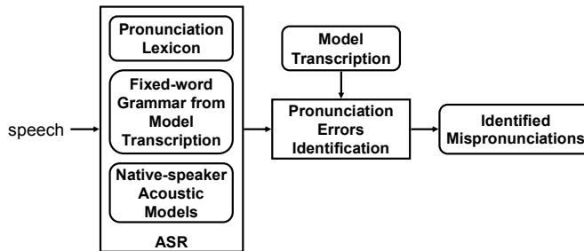
Figure 2. Schematic diagram showing the linguistically-motivated system for detecting and diagnosing L2 learners' mispronunciations.
