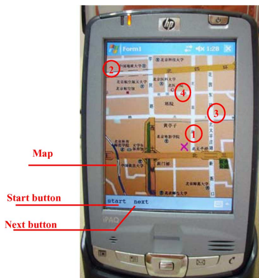
Fig. 1. Data collection interface of the Pocket PC, augmented with soft buttons for logging functions (START/STOP) and loading the NEXT map. The numbers highlight some examples of location icons: 1) subject's current location (i.e., the red cross); 2) a university; 3) a road; and 4) a hospital.
