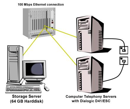
Figure 4: The telephone server setup for corpora data collection.
