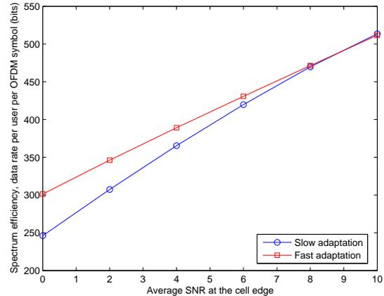
Fig. 6. Comparison of spectrum efficiencies of slow adaptive OFDMA and fast adaptive OFDMA under Nakagami fading channel with  $m = 2$ .
