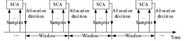
Fig. 1. Sampling procedure in the proposed slow adaptive OFDMA scheme.
