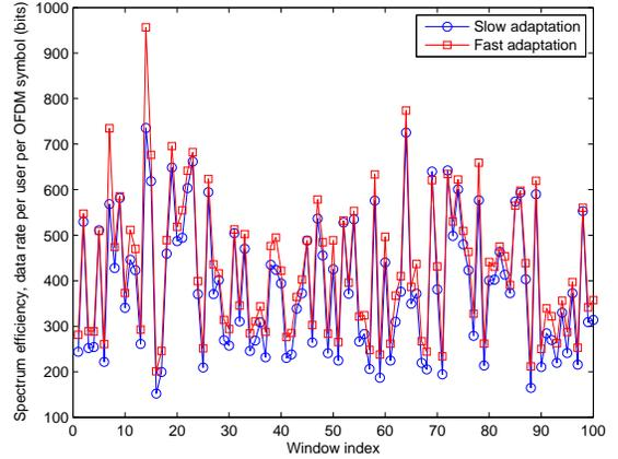
Fig. 2. Comparison of spectrum efficiencies of slow adaptive OFDMA and fast adaptive OFDMA under Rayleigh fading channel.
