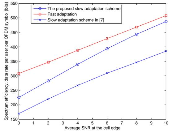
Fig. 3. Comparison of spectrum efficiencies of slow adaptive OFDMA and fast adaptive OFDMA under Rayleigh fading channel.
