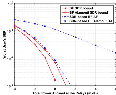
Fig. 11. Worst user's BER achieved by different AF schemes versus total power threshold in the distributed relay network:  $L = 8$ ,  $G = 2$ ,  $M = 12$ ,  $\sigma_{\text{ant}}^2 = \sigma_{\text{user}}^2 = 0.25$ . A rate- $\frac{1}{3}$  turbo code with codeword length 2,880 is used.
