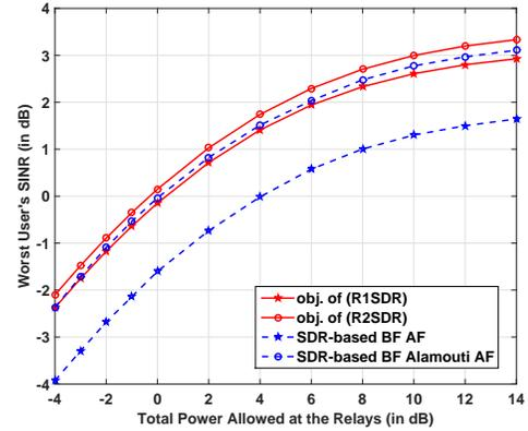
Fig. 4. Worst user's SINR versus total power threshold in the distributed relay network:  $L = 8$ ,  $G = 2$ ,  $M = 12$ ,  $\sigma_{\text{ant}}^2 = \sigma_{\text{user}}^2 = 0.25$ .
