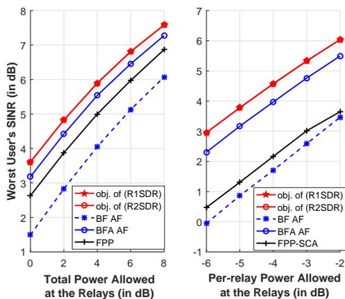
Fig. 10. Comparison with the Feasible Point Pursuit method.
