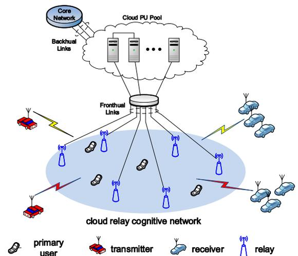
Fig. 1. An example of the cloud relay network.
