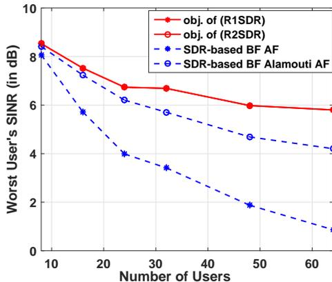
Fig. 9. Worst user's SINR versus number of users in a multicast distributed relay network:  $L = 8$ ,  $G = 1$ ,  $M = 16$ ,  $\bar{P}_0 = 10\text{dB}$ ,  $b_u = 3\text{dB}$ ,  $\sigma_{\text{ant}}^2 = \sigma_{\text{user}}^2 = \sigma_u^2 = 0.25$ .
