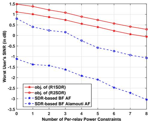
Fig. 6. Worst user's rate achieved by different AF schemes versus number of per-antenna power constraints in the distributed relay network:  $L = 8$ ,  $G = 2$ ,  $M = 16$ ,  $\bar{P}_0 = 7\text{dB}$ ,  $\bar{P}_\ell = -5\text{dB}$  for  $\ell = 1, \dots, L$ ,  $\sigma_{\text{ant}}^2 = \sigma_{\text{user}}^2 = 0.25$ .
