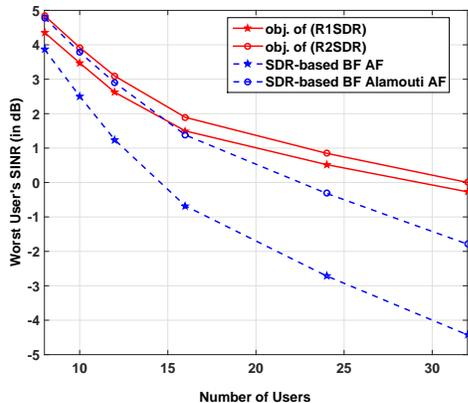
Fig. 5. Worst user's SINR versus number of users in the distributed relay network:  $L = 8$ ,  $G = 2$ ,  $\bar{P}_0 = 10\text{dB}$ ,  $\sigma_{\text{ant}}^2 = \sigma_{\text{user}}^2 = 0.25$ .
