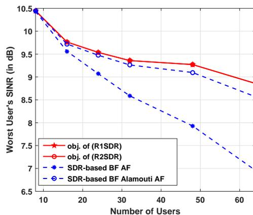
Fig. 8. Worst user's SINR versus number of users in a multicast MIMO relay network:  $L = 4$ ,  $G = 1$ ,  $M = 16$ ,  $\bar{P}_0 = 10\text{dB}$ ,  $\eta_u = 3\text{dB}$ ,  $\sigma_{\text{ant}}^2 = \sigma_{\text{user}}^2 = \sigma_u^2 = 0.25$ .
