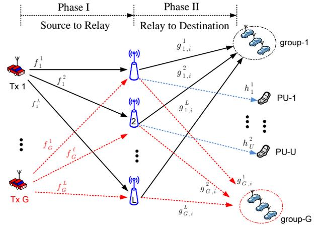
Fig. 2. The two-hop one-way relay network with primary users.
